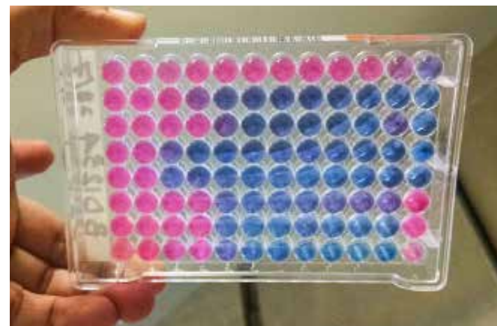
Fig. 4.1: Commercially available colourimetric broth microdilution assay, YeastOne Sensititre®, for antifungal susceptibility testing of Candida and Cryptococcus species. Growth of yeast in the wells changes the colour of alamar blue to pink, making MIC reading easier.
